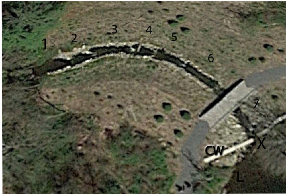
Fig. 1. Plan view of fishway showing reaches 1-7; CW= cutoff wall, L = temperature/depth logger location, and X is location of video camera.
