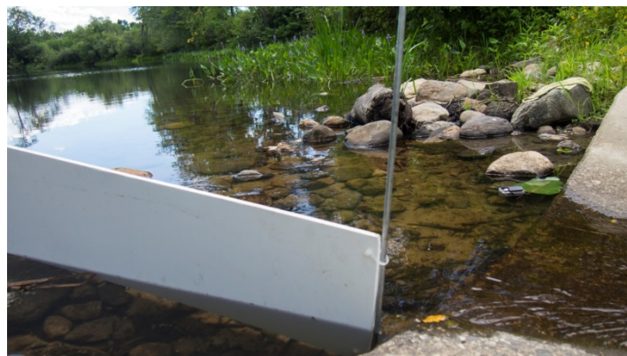
Fig. 3. White wall and camera setup for video monitoring fish moving past the v-notch in the cutoff wall (bottom right corner of picture).
